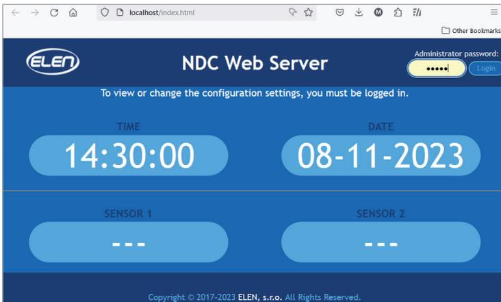
The default password „admin“ in the upper right corner is used to enter the clock configuration parameters setting. The password can be changed later in the admin menu.
