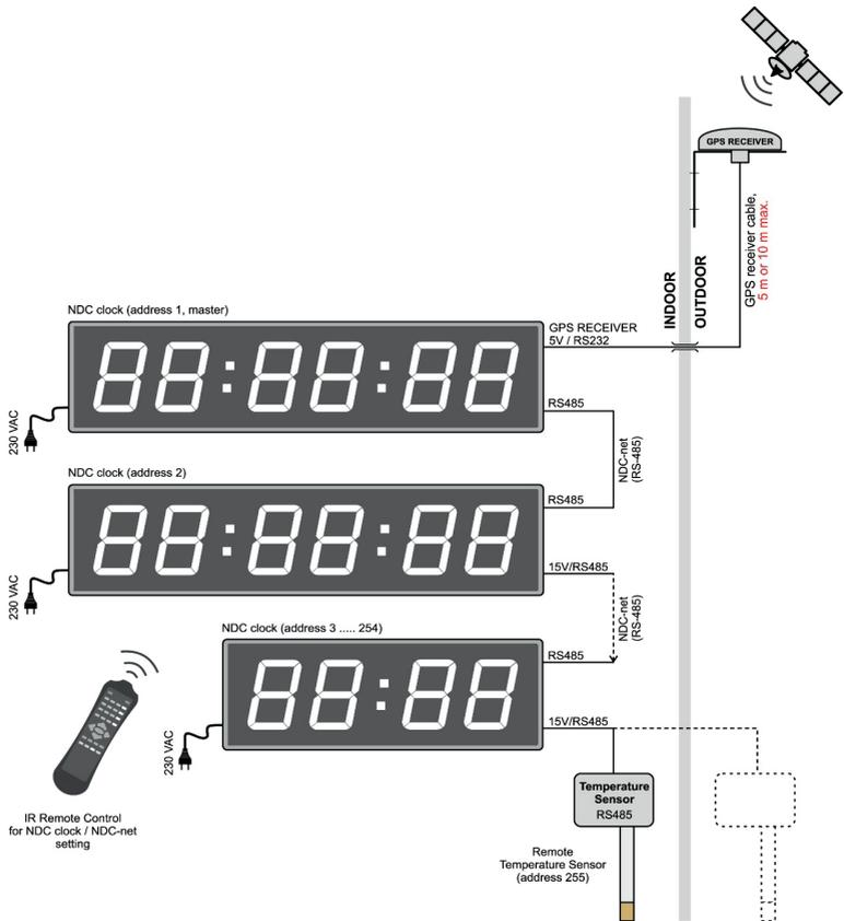
Fig. 1 Connection of NDC displays in a communication network
