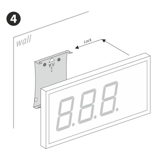
Insert display onto the mounting bracket and latch it in by moving it to the left side.
