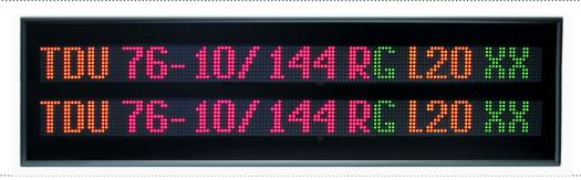
**TDU 76-10/144x2 RG L30 230AC** series alphanumeric displays are programmable electronic devices for displaying static or moving textual information.
