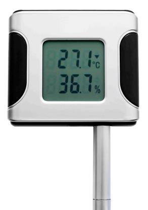
THS SENSOR 20 12DC TCP/IP is an electronic device for measuring and displaying air temperature and humidity. Its built-in LCD display provides immediate high precision reading to the user in real time. Sensor can be connected to one or more \*large-size displays on the LAN Ethernet network. External power supply adapter 230VAC/12VDC (order code KTR-0020) is required to power the sensor.
