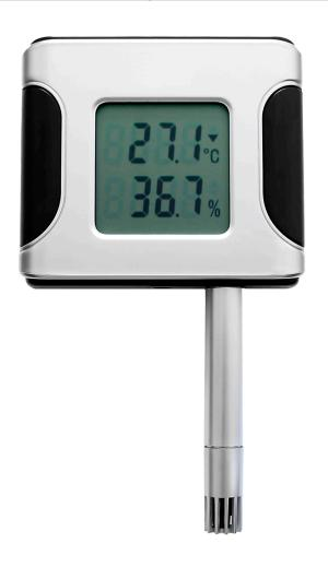
THS SENSOR 20 12DC RS485 is an electronic device for measuring and displaying the actual air temperature and humidity. Its built-in LCD display provides immediate high precision reading to the user in real time. Sensor can be connected to one or more \*large-size displays on the serial RS485 network. It can be powered directly from a large-size display, or from an external power supply adapter 230VAC/12VDC (order code KTR-0020).
