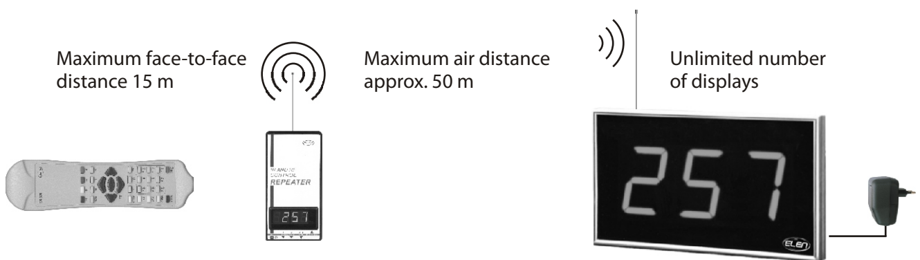
Fig. 2/ Remote control of displays from a longer distance with an IR remote control and an RF repeater
